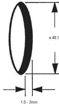
The recommended panel thickness is 1.5 to 3 mm. The drill hole must have a diameter of 48.1mm. Ensure that the installation location is level and has no sharp edges.
